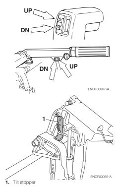
The outboard motor can also be tilted up and down using the switch provided under the bottom cowl.
