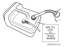
After filling the tank, close the fule tank cap.
