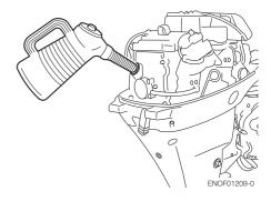
Use only high quality 4-stroke engine oil to insure performance and prolonged engine life.
