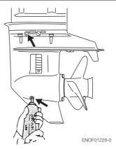
Install the upper oil plug, and then remove oil tube nozzle and install the lower oil plug. ENOW00095-0
