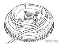
5. Tie a loop in the another end of the emergency starter rope and attach socket wrench that is included in the tool kit.
